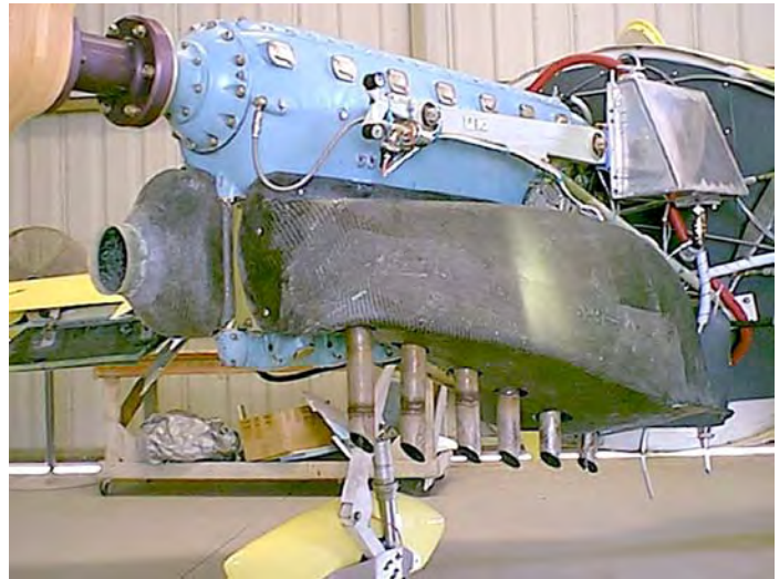
The air-cooled, supercharged, 235 HP Walter-LOM inverted inline 6 cylinder engine.
