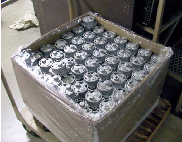
Revmaster builds their own oil pump in-house. Above is a small portion of pumps being machined. Below is a case of housings yet to be machined.
