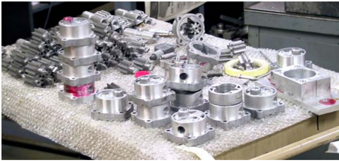
Revmaster builds their own oil pump in-house. Above is a small portion of pumps being machined. Below is a case of housings yet to be machined.
