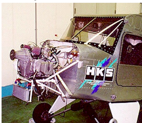
Murphy Maverick used as an HKS 700E engine test bed.
