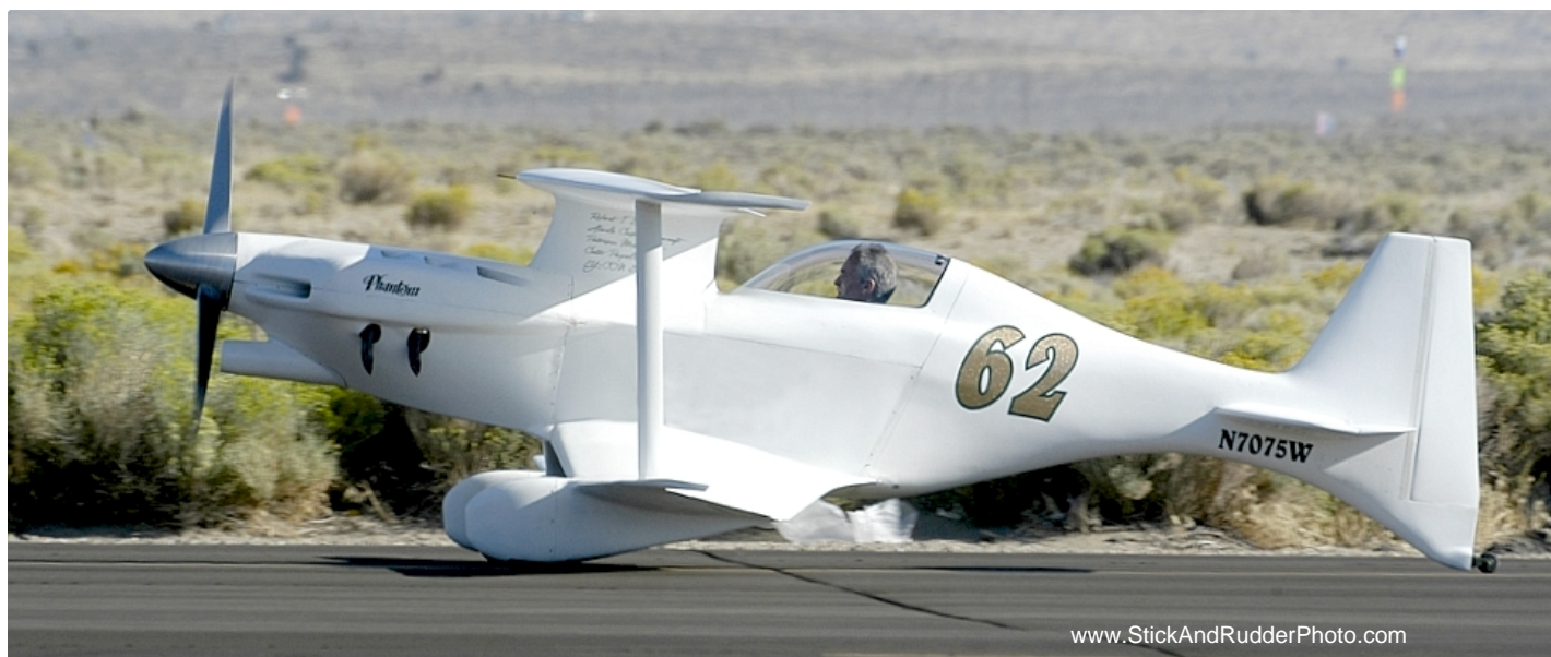
This Reno 2003 photo, shot by Chris Luvara, clearly shows the straight stack exhaust system Tom once used.
