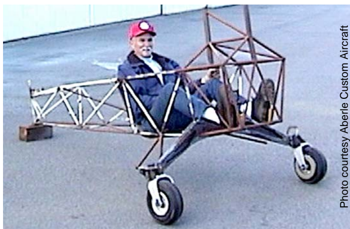
Tom test drives the Mong Sport fuselage truss before hacking off the aft section for the carbon fiber monocoque tail cone and empennage.
