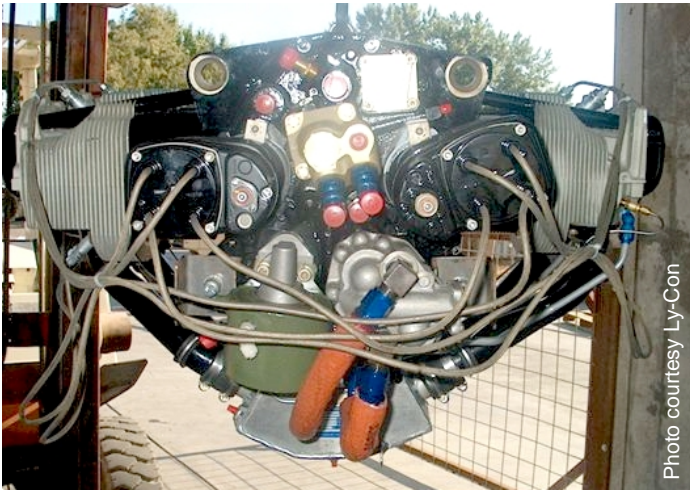
The rear view of the engine, showing a little more of the intake manifold.
