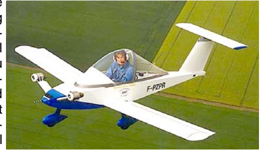
French built "Cri-Cri" has been flown with twin jet engines used in the model airplane industry
