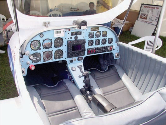
Super Pulsar 100 cockpit. Note the wide 44" shoulder room and full IFR panel.
