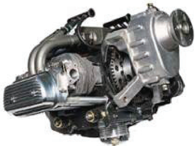
Unlike most VW conversions, the Aeromaxx engine drives the propeller off the flywheel end of the engine, not the more failure prone pulley end.
