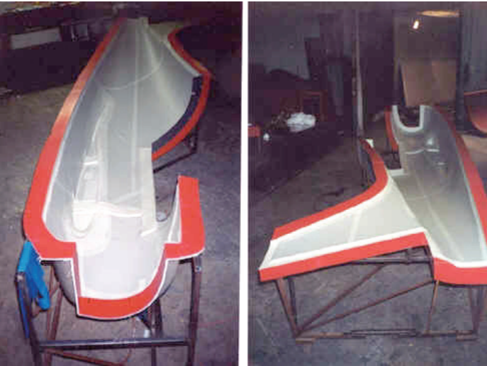
The integral vertical fin can be seen in this view of the molds, with the initial layers of pre-impregnated cloth in place.
