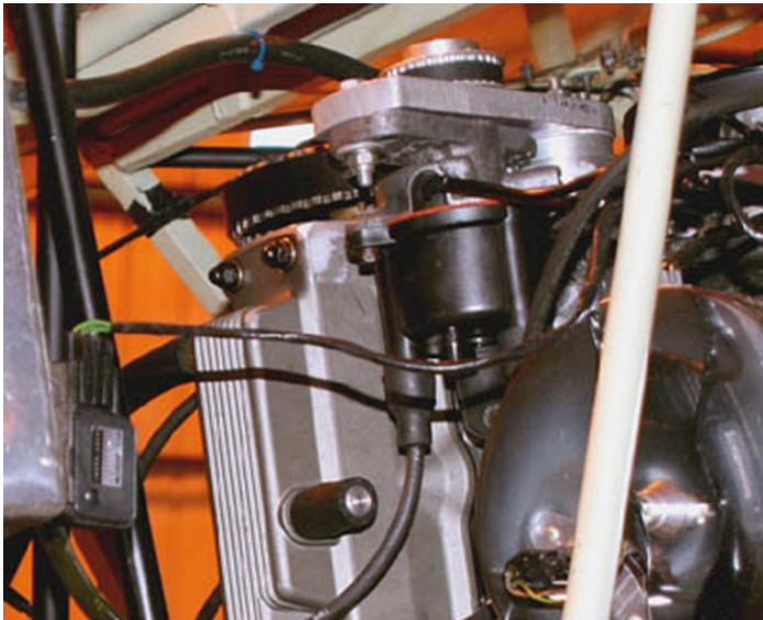
With the Geo distributor normally directly driven off and inline with the camshaft, Lyle had to adapt its operation from the side in order to fit everything within the confines of the fuselage. Larger view
