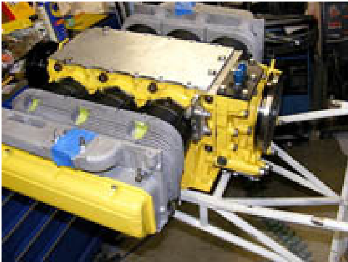
The long block installed before any accessories
