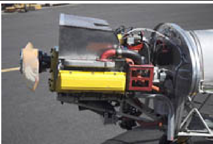
Temporary cooling air plenum in place for initial test runs
