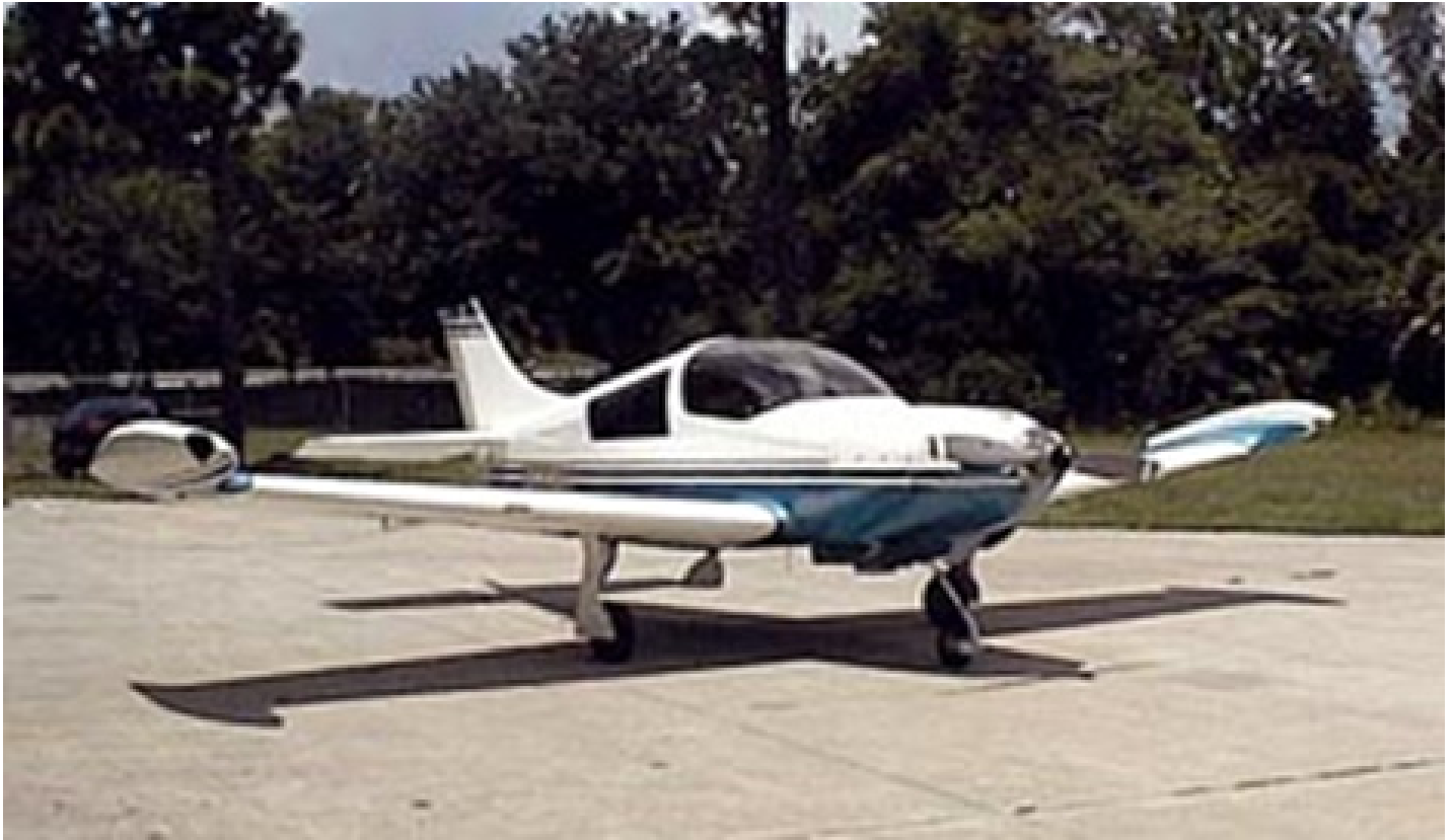
A two place Cavalier experimental airplane using Cessna-style tip tanks Photo: Karl Walter
